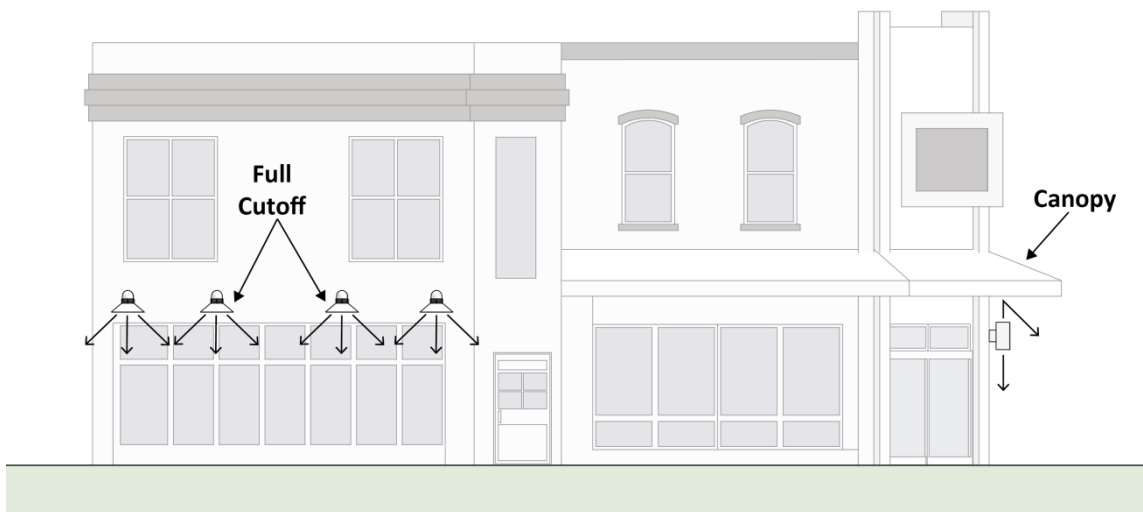
Figure 52: Exterior Light Shielding
